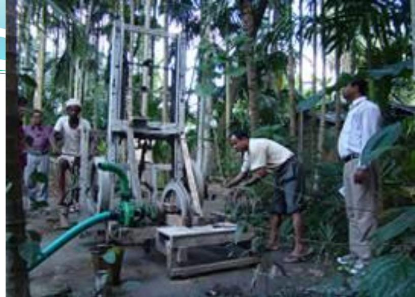
**Testing of paddle operated pump**
